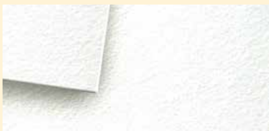
HGT - Glazed surface for fine dust and increased cake release
