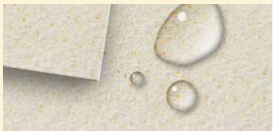
TF - Fluorocarbon with PTFE resins heavy finish for increased water and oil repellency and difficult agglomerating dust
