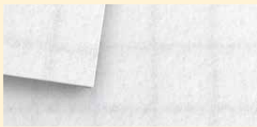
PE AGT BT - Polyester needlefelt on antistatic stainless scrim support
