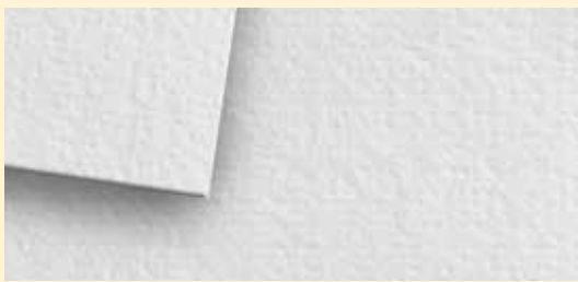
H2T - Working and clean side singed surface for better mechanical properties and easier cake release
