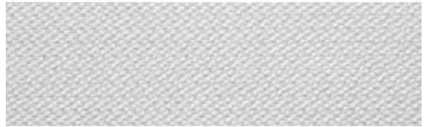
PP 50 (100% polypropylene, warp-multifilament, weft-yarn) Applications: galvanic, waste water
