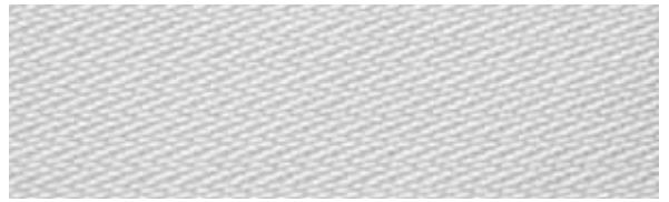
PP 41/V (100% polypropylene, warp-multifilament, weft-yarn) Applications: wine bags
